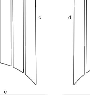
Installation Note: Graphic kit is designed so that the top of each graphic panel is installed at the bottom of each body side indentation, centered.
